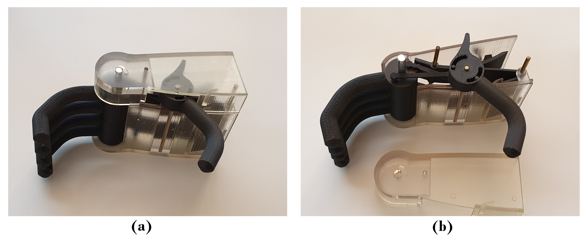
Figure 3: Second 3D-printed polymer replica of the first "Iron Hand" of Götz von Berlichingen with an improved thumb lever mechanism. (a) General view of the artificial prosthetic hand; (b) view after removal of the lateral chasis cover with insight into the new mechanics.
